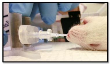
Figure 1: Rat intranasal catheter device.
