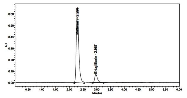
Figure 2(a): Chromatogram of standard solution.
