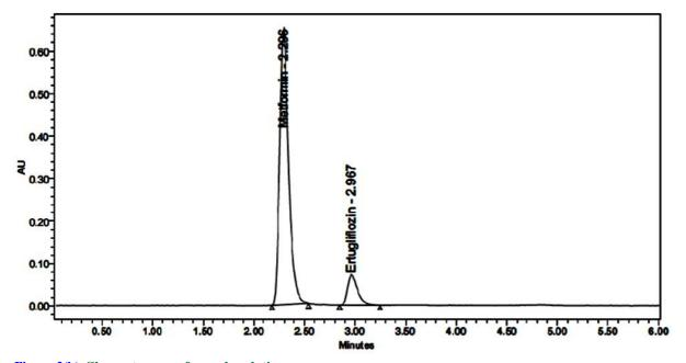
Figure 2(b): Chromatogram of sample solution.
