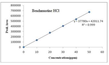
Figure 5: Calibration curve of linearity.
