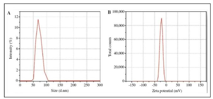
Figure 3: (A) Size distribution potential and (B) Potential distribution of synthesized ZnO-NPs.
