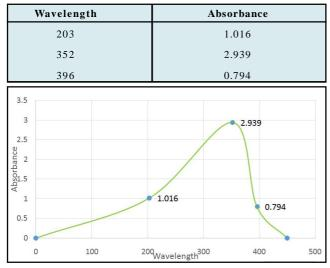
Figure 5: Spectrum of ZnO-NPs synthesized by green method.
