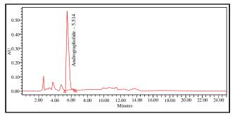
Figure 2a: Chromatogram of methanol extracted sample of AP.
