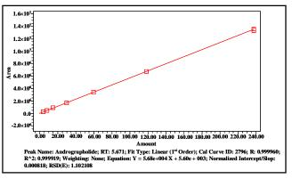
Figure 3: Calibration curve of andrographolide (Reference compound).
