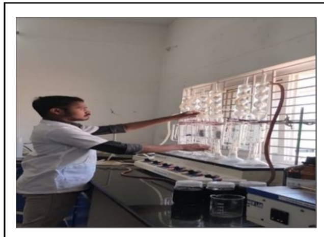
Figure 5: Alkaloids extraction of powdered mulberry leaves samples using methanol.
