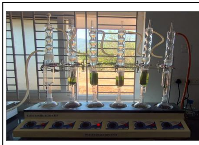
Figure 6: Soxhlet extraction for GC-MS analysis.
