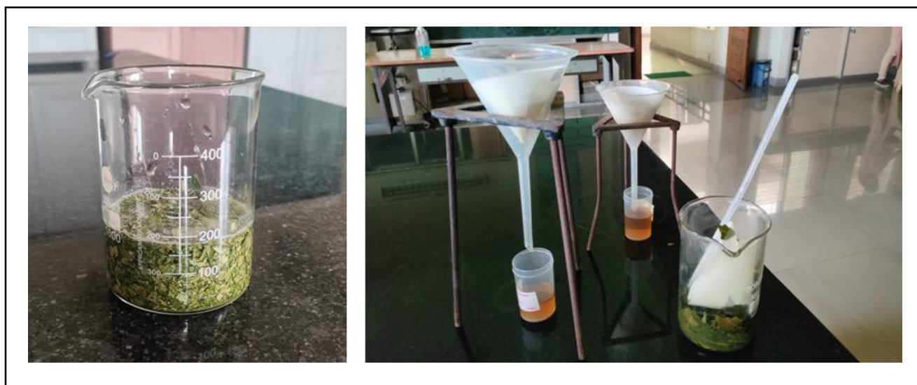
Figure 1: Preparation of aqueous neem leaf extract.
